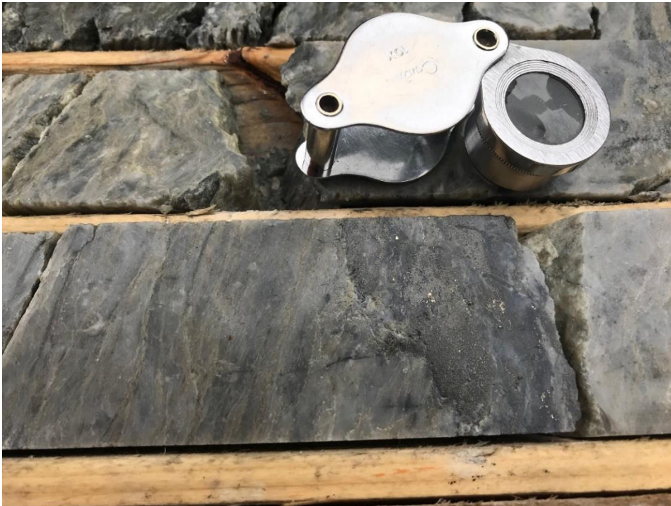
Figure 2: Core photo of GA-20-35 displaying visible gold ( click image to enlarge )
